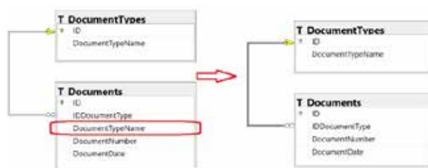
Fig. 4. Database diagram with/without redundant attribute
